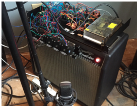
Figure 2. Arduino and stepper motors configured for control of a Fender Princeton Reverb amplifier.
