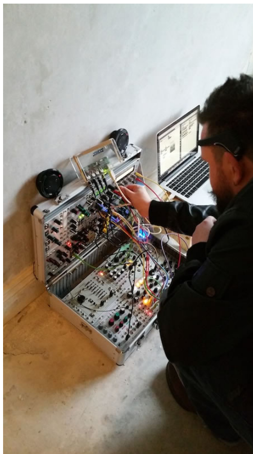
Figure 1. Dave O Mahony's setup consists of an Interaxon Muse Headband (brainwave sensor), a Eurorack system and a computer interface.
